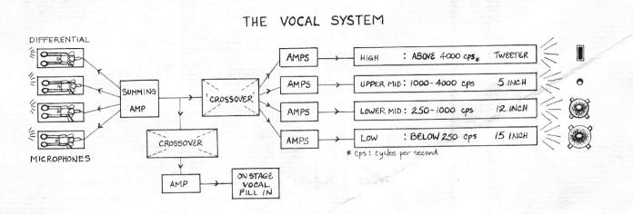
The center cluster of the vocal system, consisting of high and midrange speakers, is curved so as to disperse sound cylindrically; there is not much vertical dispersion, and horizontal dispersion is ideally between 140 and 180 degrees. The vocal low range speakers are arranged in a column. Each type of speaker is designed to have the same horizontal and vertical angle of dispersion so that all frequencies are heard equally well.
